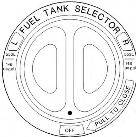
Figure 7.7.2 - Manual selector of fuel tanks
