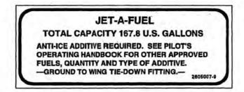
12. Adjacent to each inboard fuel tank filler cap (when installed):
